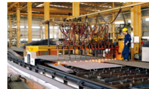
Cutting Production Line 切割生产线
